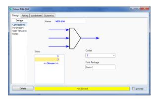
The status bar should be yellow. This indicates that the block has not been calculated.
