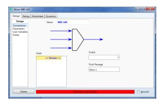
Locate the *Inlets* area on this dialog and click in the first cell. Select stream "1". Repeat for stream "2".
