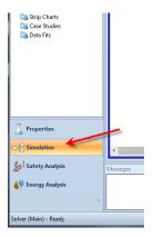
As you click this button Aspen HYSYS temporarily passes control to the OLI software to create the electrolyte model. Progress messages can be seen in the status line at the bottom of the window as well as in the summary box. After a few moments, the standard ASPEN HYSYS development window is displayed.
