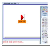
The mixer is given a default name of MIX-100. You can change it later if you wish. The block is also colored RED. This indicates that the block does not have sufficient information to calculate.
