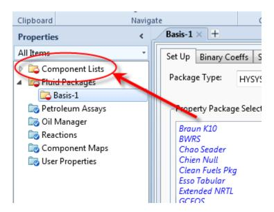
Click the small arrow to expand the list. This will expand the list to display all the component lists.
