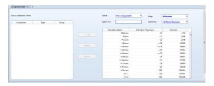
Aspen HYSYS categorizes the components according to function and type. OLI Components are no different. Expand the drop-down list from the *Select* box.
