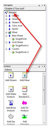
We can now add the "Base Waste" and "Acid Waste" stream as we have done in previous examples. The only difference here is that we are selecting an **Adiabatic** calculation instead of the default isothermal calculation.
