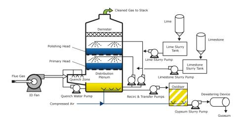
The application is modeled in ESP using a multi-stage absorber, a sparging tank, mixers, pumps, filters, controllers, and recycle-stream calculators.
